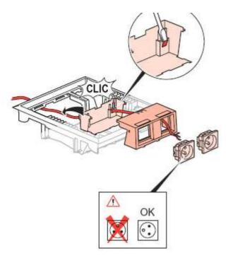
Be careful when positioning sockets in their supports. (earth electrode on top = side outlet plugs can't be used)
